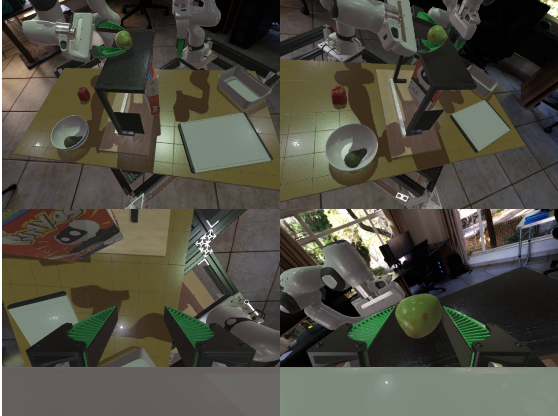
Figure 16 Example of sensor measurements at inference time. Image captured at approximately the same timestamp as the PlaceAppleFromBowlIntoBin render in Figure 6. The images are then post processed further for input to the VLA models such as FOUNDRY-QWEN3VLA-2.1B and FOUNDRY-VLA-1.7B. While some simulation stations include an extra wrist camera per arm, FOUNDRY-QWEN3VLA-2.1B and FOUNDRY-VLA-1.7B use only the four shared cameras for VLA training and inference. Refer to [65] for further details on the simulation stations.
